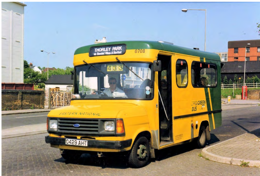
Smallest minibuses in the EN fleet were the 16-seat Ford Transits like 0708, which had been new to Bristol Omnibus Co and moved to EN in summer 1990. The Carlyle-converted Dormobile bodies only had a single destination aperture so three-track number blinds were fitted behind the windscreen. Seen at the Bishops Stortford Interchange. EBEG collection
