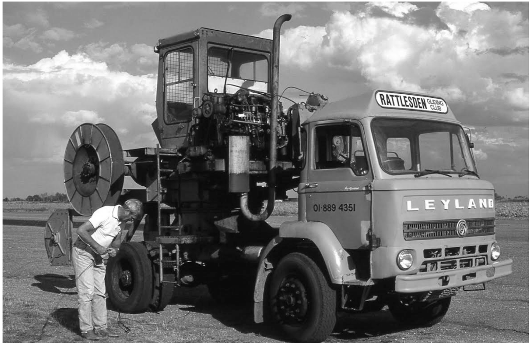
Photo above: Some years later, (August 1996) the engine and gearbox still remained, powering the glider winch on the back of a truck - apparently semi-autos are favoured for this task, presumably as they are more controllable. Gary Sharpe.
