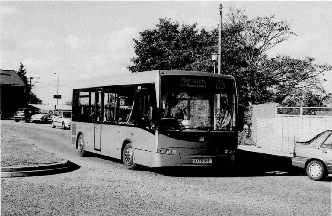
Plaxton Primo demonstrator YX55 DSE at on the 22A/B Harwich town service: above, with the High Lighthouse in West Street; and, below with Harwich Town rail station in the background. The Primo is a 7.9m long, 2.4m wide 28-seater, with Cummins ISBe Euro 3 engine and Allison gearbox. The chassis is built by EBL in Hungary and the body at Scarborough. An unusual feature is the pivoted, single-leaf, coach-style door. Fred Lawrance
