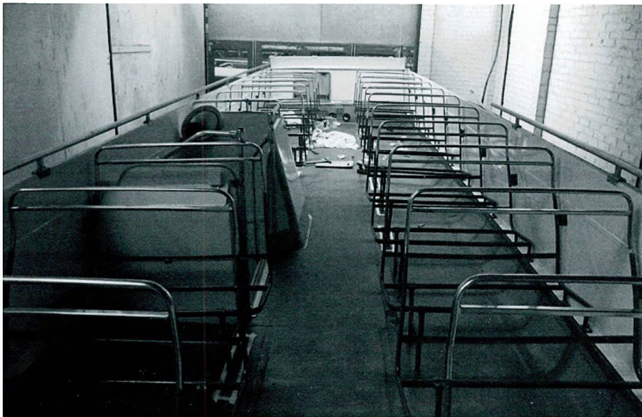
May 2012: Top-deck prepared and painted with red oxide waterproof paint, sidewalls painted cream, and seat frames (repainted blue) installed. Seat handrails await application of chrome polish (+ elbow grease). Seat squabs yet to be refitted. Ian Banks
