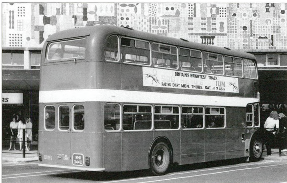
This view of 2859, RHK344D in Basildon Bus Station shows off the characteristic rear of the FLF with its central emergency door which was not entirely successful in the quest to keep Doug's conductor where he should be!
