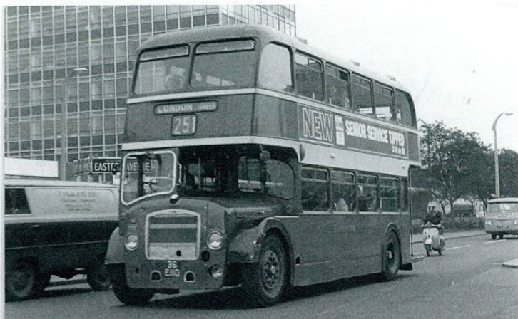
1484 (latterly 2453 ) - 36 ENO a 1955 Bristol LD6B on Eastern Avenue Gants Hill heading for Wood Green on the 251 with some nice period Ford and Commer vans. It was taken a while into its life as the 3 piece destination has been replaced with the Tilling "T" style destination without intermediate displays, but before the 1964 re-numbering. Lyn Watson.
