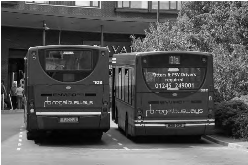
Regal's 702 and 652 parked at Chelmsford Bus Station on 21 August show the difference in rear bodywork between an Enviro 200 on a MAN chassis (702) and on an Enviro 200 Dart chassis (652).
