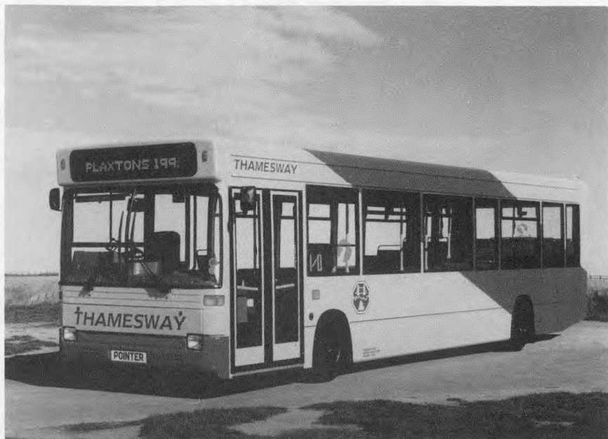
Photo: Thamesway 701 is the prototype 9.8m Dennis Dart SKF low floor bus with Plaxton Pointer bodywork. photo - Plaxton
