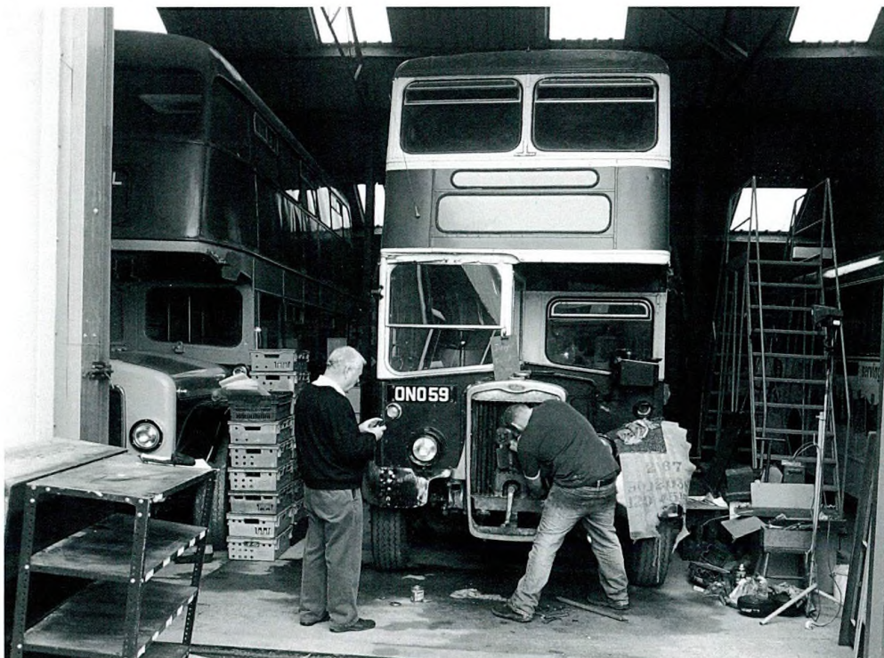
Earlier in 2013, work was taking place on ONO's radiator in the LVVS workshops.
