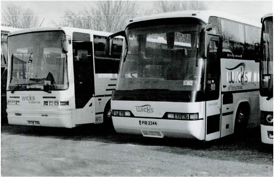
Two Dennis Javelins with contrasting styles of bodywork are seen here. PIB 2344 has a Neoplan body whilst R719 TRV has a much more restrained UVG coach body.
