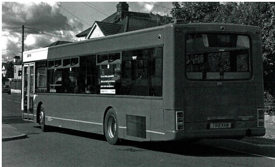
Freshly repainted DAF SB220 / Plaxton 3918, T918 KKM, at Shoebury on 30 September, illustrates the box-like Prestige bodywork and the (unused) rear number indicator suspended from the internal roof panelling. John G Lidstone
