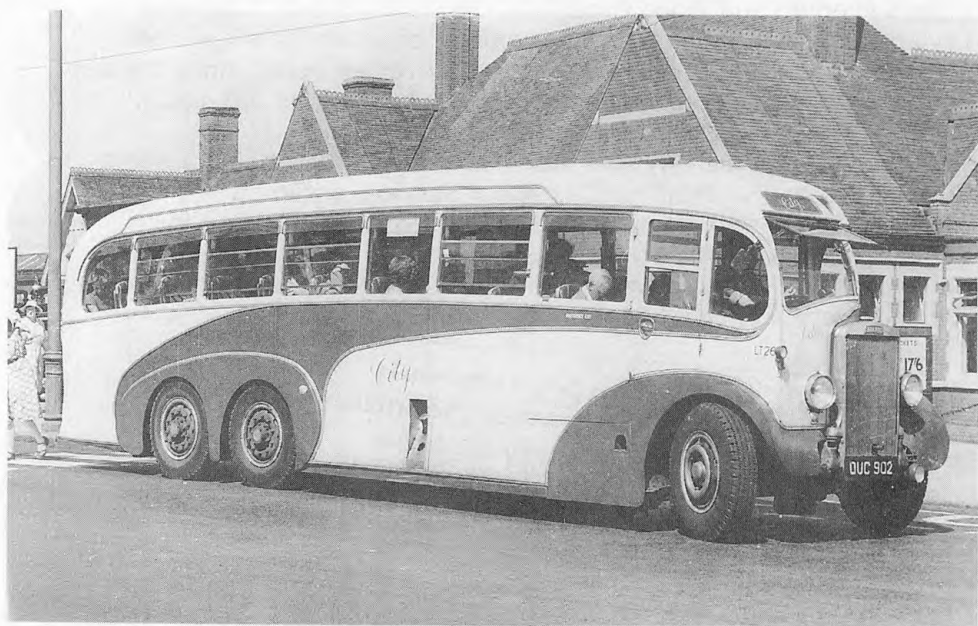
Six-wheeler Leyland Tiger LT26 (DUC 902) is seen outside Southend Victoria Station. The vehicle was delivered in 1936 and was fitted with a new Heaver centre entrance body in 1947. (F. Church)
