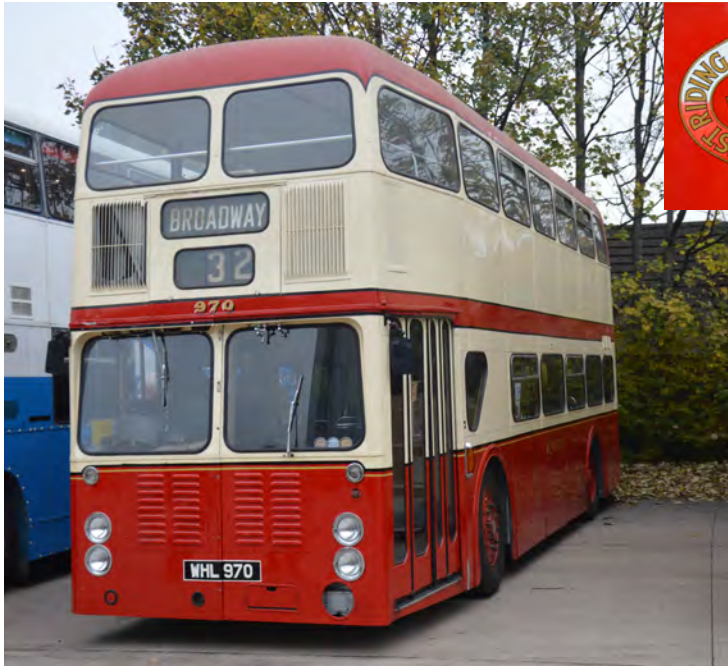
Inward camber on the front wheels led to very short tyre life.
