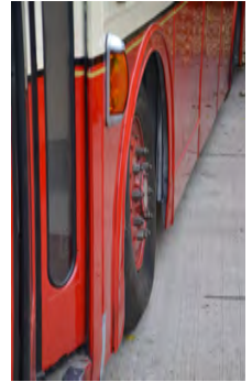
Inward camber on the front wheels led to very short tyre life.
