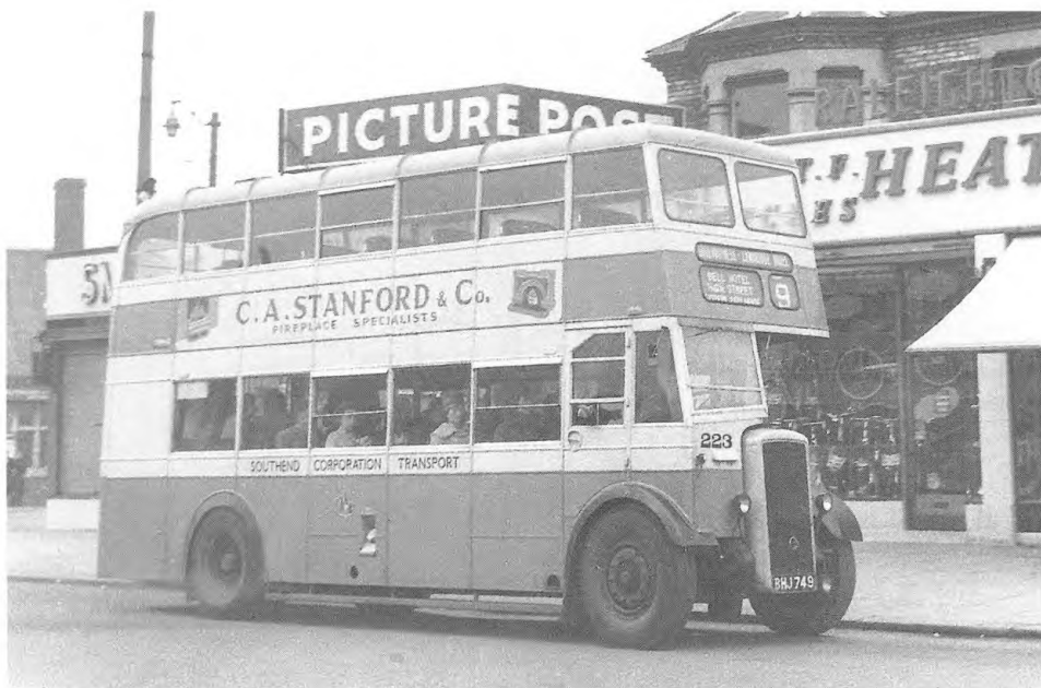
Southend Corporation 223 (BHI 749) Daimler CWA6/Duple , seen in post-war years heading for Shoeburyness. Apart from receiving upholstered seats, rubber-set top-deck front windows and the postwar standard Southend destination layout, the utility body appears to be unaltered. 223 was sold and scrapped in 1958. Brian Pask
