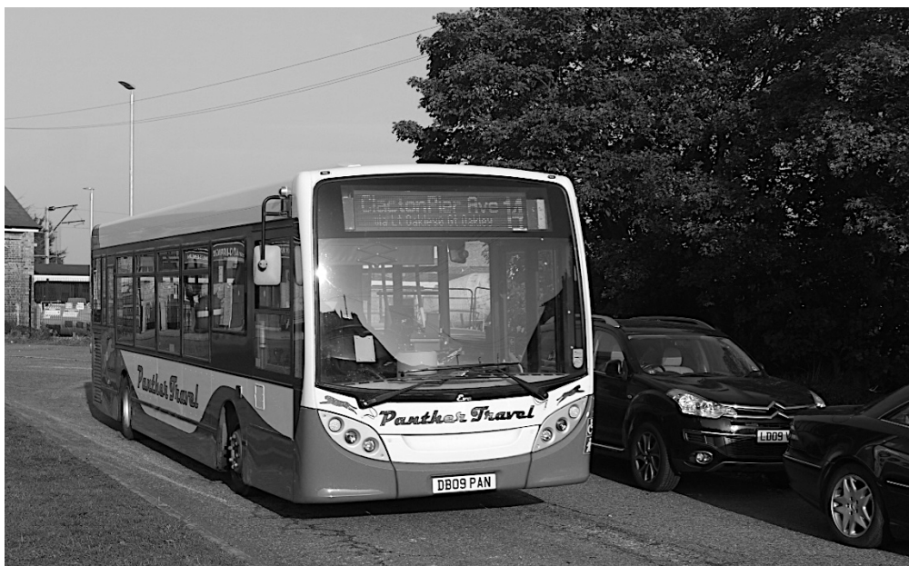
Lower picture Panther Travel DB09 PAN (YX09 AEV) ex Metroline Alexander Dennis Enviro 200, departing from Harwich on 0925 service 14 to Clacton on 16 October 2018. Rebuilt by Panther Travel from B29D to B36F and repainted by Mardens of Benfleet. No trace of where the second door was.
