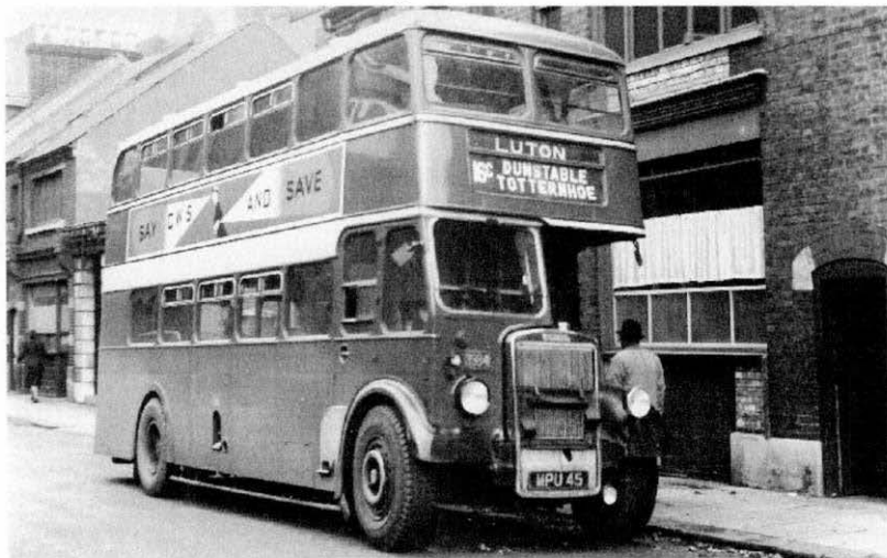
3984 (MPU 45), one of the Midland Area Luton allocation. The bus, with its adjustable radiator muff in place, and passers-by in hats and coats suggest this is wintertime. Photographer unknown
