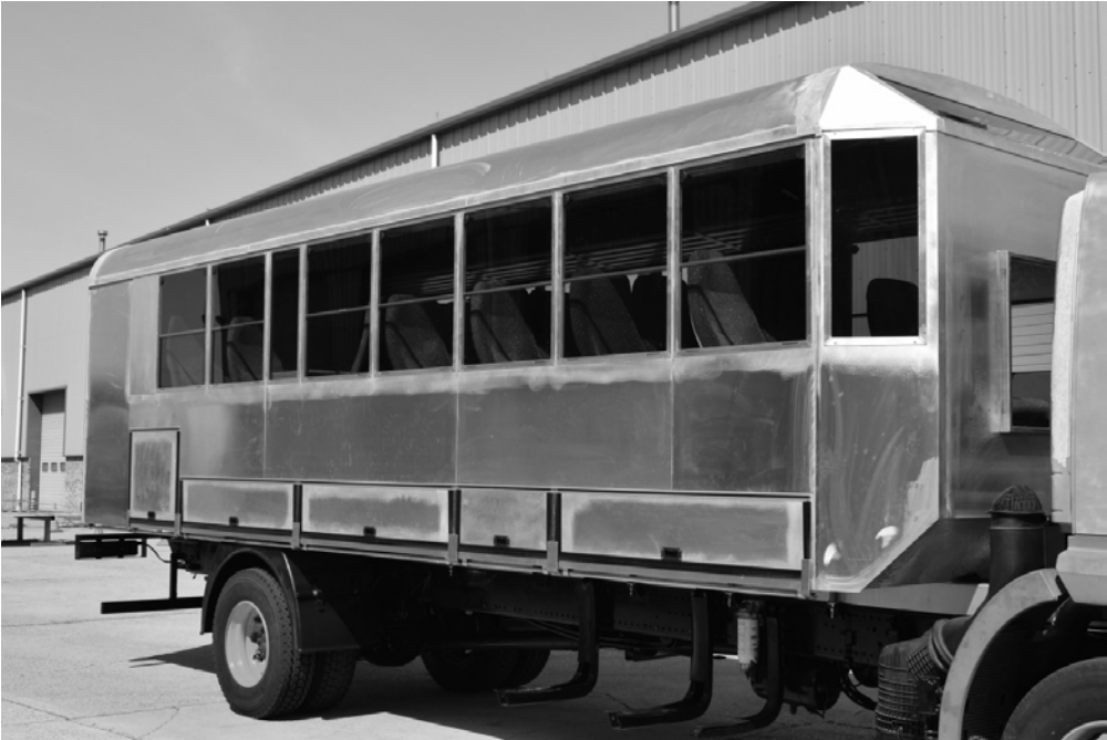
Picture previous page Body in build at ASGB Frating July 2018, the under floor lockers visible, looking at the rear offside corner with wood cage and two spare wheels yet to be fitted to the rear bodywork. Mark Lloyd. EBN653p24
