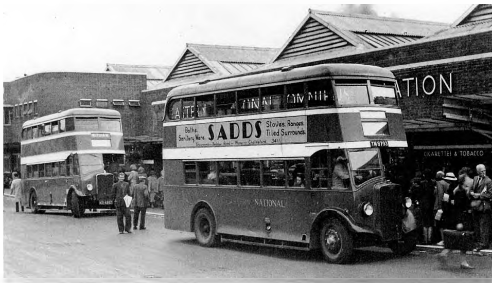
below: A busy, just-postwar scene: 'EASTERN NATIONAL OMNIBUS STATION' in Tilling-style lettering on the brickwork. 3077 (TM 8793), a 1931 AEC Regent with Stracham body rebuilt by Beadle in 1944. It was scrapped in 1955. Behind, loading for Witham, is 3437 (KR 4997), another Regent, but with Short body, new to Borough Services in 1930 (and possibly a former Shorts demonstrator). It was rebuilt by Beadle in 1947, and survived until 1956 (as 1149). both: Omnibus Society
