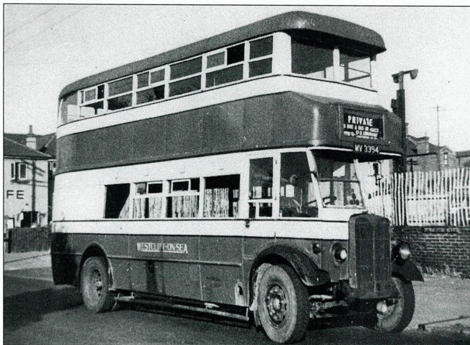
One of the oldest buses seen by Terry Challis in his Hadleigh childhood was Westcliff MV 3394, a 1931 built AEC Regent with distinctive Metro-Cammell "piano front" body. It was originally an AEC demonstrator and appears to have a London style straight staircase. It is seen here late in its life outside the Westcliff MS Prittlewell garage and works in Fairfax Drive. EBEG collection
