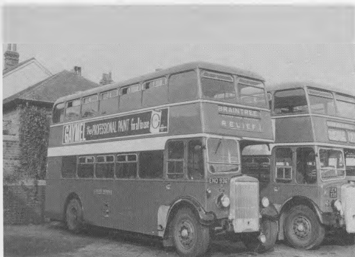
Braintree Bus Park is the location of this view of one of the more venerable members of the fleet. Leyland TD4 1107 (ENO 936) was new in 1937 as 3658 with an E.C.O.C. L24/24R body. After being rebuilt by Beadle, rebodied by E.C.W. and re-engined by Gardner it survived until 1963.
