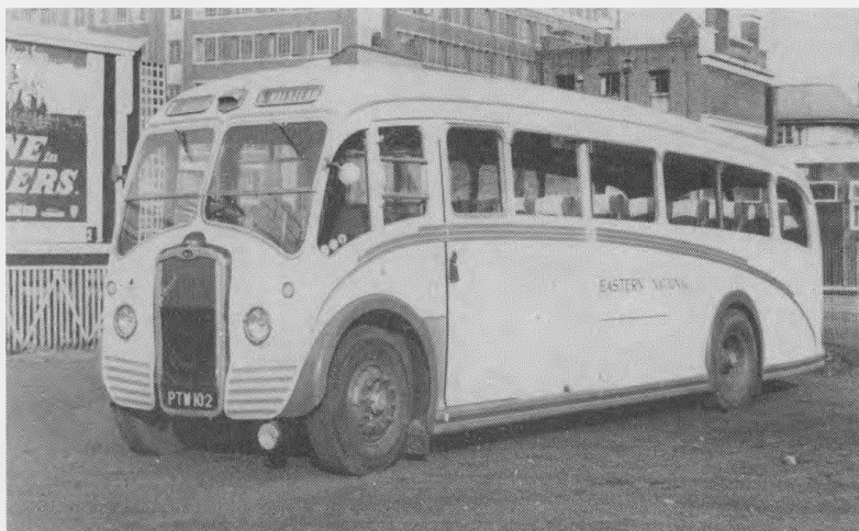
Seen at the Euston Square terminal in London on express service 'B' to Halstead is 320 (PTW 102) a Bristol L6B with E.C.W. FC31F bodywork dating from 1950.
