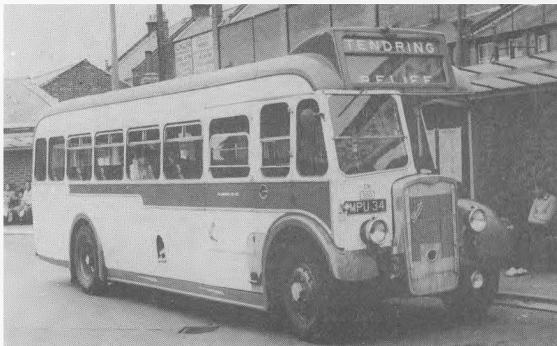
Clacton Bus Station is the scene for this view of 300 (MPU 34), a Bristol L5G with 31-seat E.C.W. dual purpose bodywork about to depart for Tendring Hospital. These vehicles were regular performers on the express services from London carrying loads of happy holidaymakers to the Butlins Camp.
